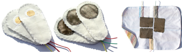
Fig. 5. Test patches and blanket
